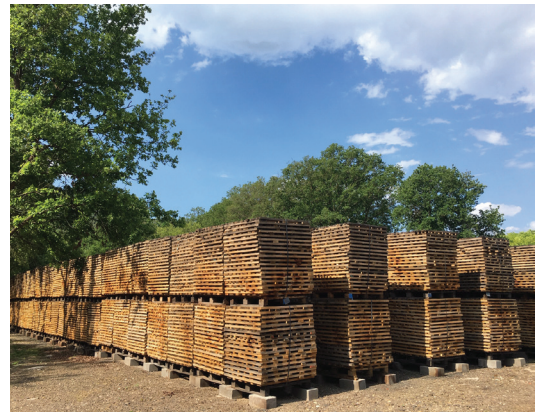
Stave Seasoning Yard
